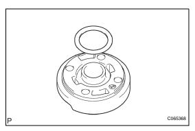
(b) Coat a new O-ring with power steering fluid and install it onto the side plate.
