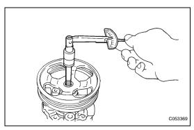
(c) Using a torque wrench, check the pump rotating torque.
